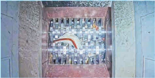
Low-speed rotary crushing machine Wooden furniture and other items are crushed into small pieces by two blades that rotate in opposite directions.
