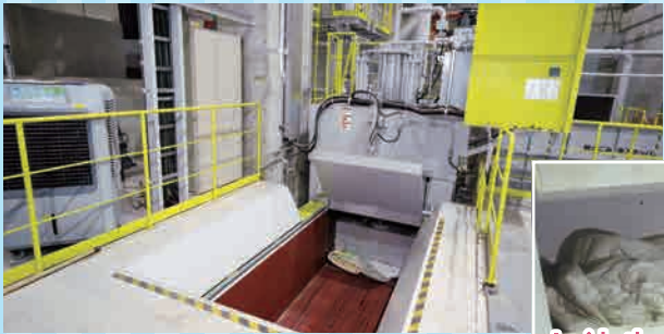
Vertical cutting machine Soft, large-sized burnable waste such as tatami mats and futons are cut into fixed lengths with powerful blades.
